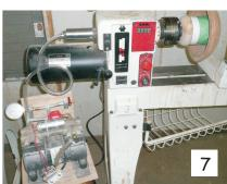
True up foam pad mating surface (use negative angle rake scraper on plastic, suggest skew chisel, laid flat on tool rest.
